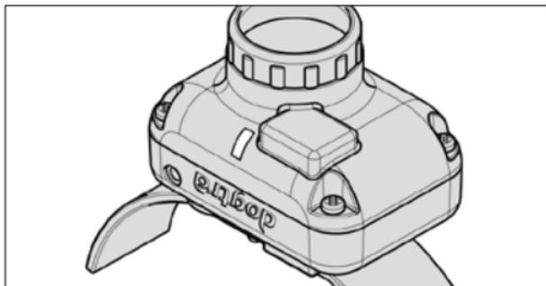
Located on the front of the STB BEEPER COLLAR, the LED indicator flashes every 4 seconds when the receiver is on and ready for use.
