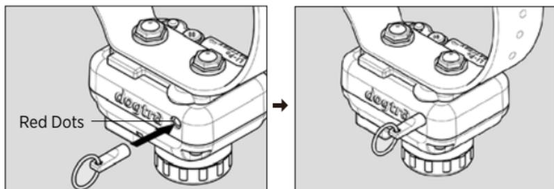
To turn on the STB BEEPER COLLAR, place the activation magnet on the magnetic red dot on the STB BEEPER COLLAR. Hold them together for a moment until the LED light comes on. The system will play a melody and then beep twice when it is turned on.
