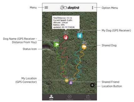
With the GPS connector paired to a GPS receiver and phone or when receiving shared GPS connector or receiver devices, the positions will be displayed on the map.
