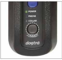
The Connect button is used to connect the GPS connector to a smartphone and GPS receiver.
