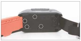
Open the antenna enclosure by removing the 4 screws and the contact points. Remove the screw holding the antenna in place to replace the antenna.
