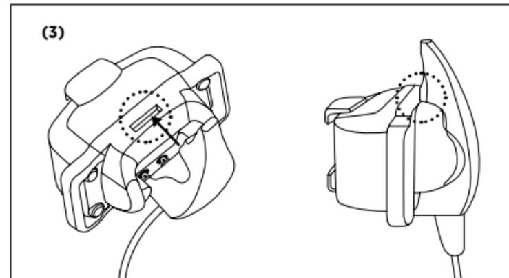
3. Push the pointed part of the charger until you hear the snap to secure the placement.
