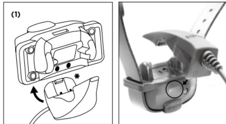
1. Place the square latch\* on the base of the charger to the LED screen notch on the receiver.
