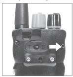
The transmitter for the T&B DUAL has seven buttons (three on the face of the transmitter, three on the left side, and one on the right). You can use the Setting Toggle Switch on the back of the transmitter to change from **T** (Training Setting) to **B** (Beeper
