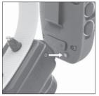
2. With the receiver turned off, place the red dot on the transmitter to the red dot on the receiver. Hold the two red dots together until the green LED blinks rapidly on the receiver. When the receiver light blinks rapidly, separate the two devices.
