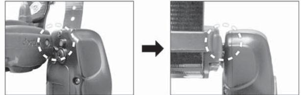
To activate the receiver/collar, place the red dot on the back of the transmitter to the red dot on the receiver/collar. Hold the two red dots together for a moment until the LED light on the receiver/collar comes on.
