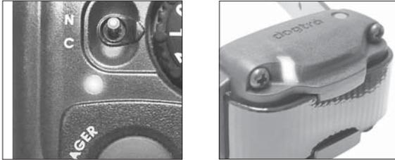
The LED indicator color indicates the battery life level. **Green** = Fully charged, **Amber** = Medium, **Red** = Needs charging
