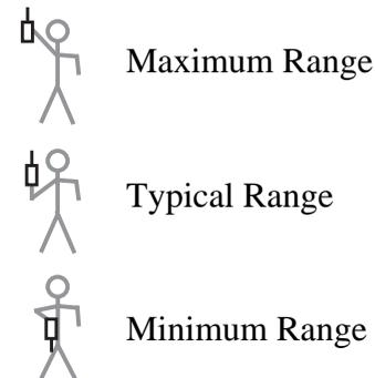
If your finger touches the antenna near the dial on the top of the transmitter, the actual range may be reduced. Additional environmental factors may also affect the range of your unit.
