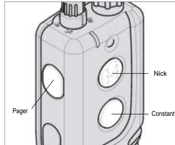
The transmitter for *dogtra* 1400NCP Woodgrain Finish Series has three buttons (two on the face of the transmitter and one on the side).
