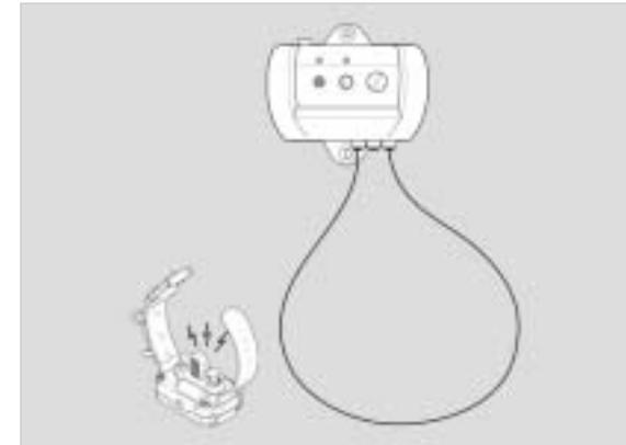
1. To ensure that your *dogtra* e-Fence System is working properly, connect the transmitter adaptor into the jack connector of the transmitter and then plug the adaptor into a household outlet. The ON/OFF indicator light should be on.
