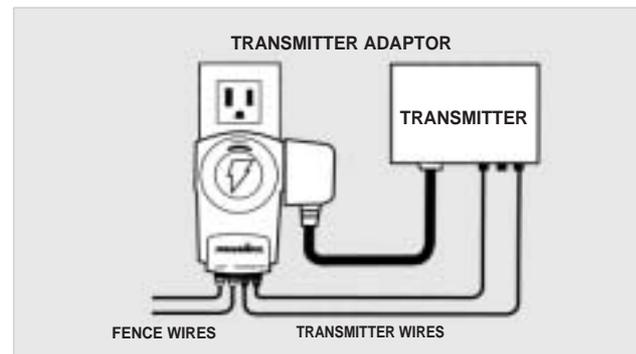
**STEP 1** Plug the lightning protector into a grounded (3-wire) 120V AC outlet within five feet of where you want to locate the transmitter
