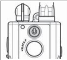
2. - To code the Black Collar set the Toggle Switch on the front of the transmitter to the “up” position.
