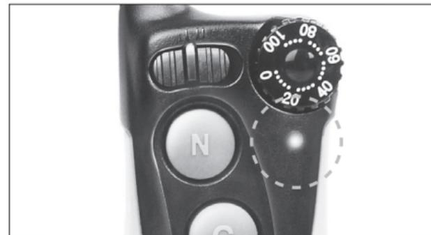
The LED indicator flashes every 4 seconds when the receiver is on and ready for use. The LED indicator will blink on both the transmitter and the receiver when the transmitter buttons are pressed.
