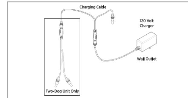
The iQ PLUS uses lithium-polymer batteries. The battery charger and charging cables allow you to charge both the transmitter and receiver at the same time. The battery charger is designed for a 120 volt wall outlet.
