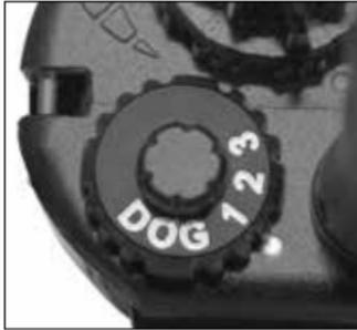
1. Set the Selector Dial to level 1 and set the Dog Selector Dial to the number you want to code the receiver to.
