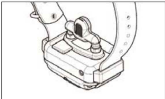
1. Turn on the receiver/collar and place the test light over the contact points as shown in the diagram.
