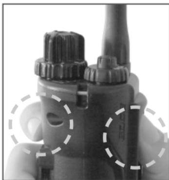
4. Within 5 seconds of separating the transmitter and receiver/collar, hold down the top orange/constant button on the front of the transmitter and the Pager button on the back of the transmitter at the same time. The code setting is complete when the LED indicator resumes blinking every 4 seconds on the receiver/collar.
