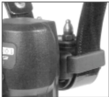
2. With the receiver/collar turned off, hold the red dot on the front of the transmitter to the red dot on the receiver/collar for about 5 seconds.
