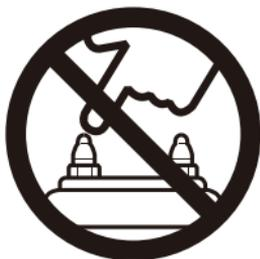
3. **IMPORTANT!** Place the receiver/collar aside when the LED indicator rapidly blinks green on the receiver/collar. Take caution not to touch the contact points on the receiver/collar during step 3 or you may receive an electric stimulation.
