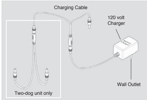
The battery charger and charging cables allow you to charge both the transmitter and receiver at the same time. The battery charger is designed for a 120-volt wall outlet (European 230-volt AC chargers and 10-volt field charger for Lithium-Polymer batteries for your automobile are also available.).
