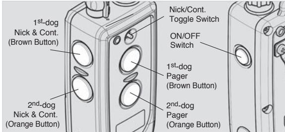
The **dogtra 2302NCP Advance** two-dog unit has five buttons and a toggle switch on the transmitter. Two on the face of the transmitter, two on the left side, and one on the right side.
