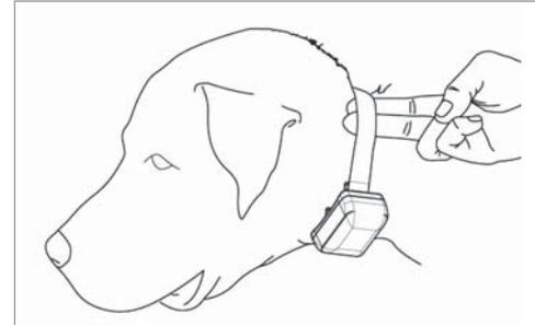
The collar should be fitted so that the surgical stainless steel contact points press firmly against the dog's skin. You should be able to fit a finger in between the contact point and your dog's skin.
