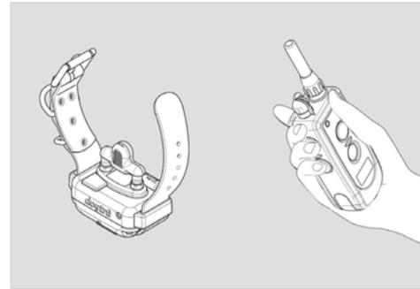
1. To activate your *dogtra* 2300NCP Advance Series place the red dot on the back of the transmitter to the red dot on the receiver/collar. Hold the two red dots together for a moment until the green colored LED indicator light comes on.
