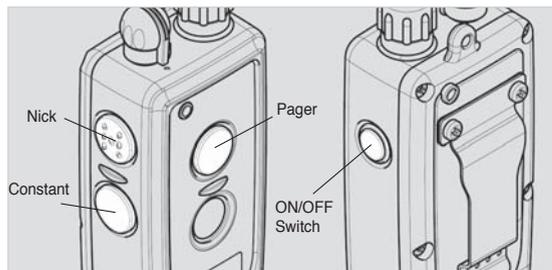
The transmitter for the *dogtra* 2300NCP Advance single dog unit has four buttons (one on the face of the transmitter, two on the left side and one on the right side).
