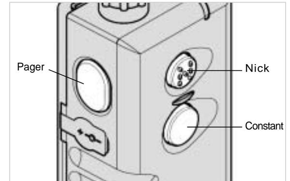
The transmitter for *dogtra* 180NCP Woodgrain Finish has three buttons (two on the face of the transmitter and one on the side).
