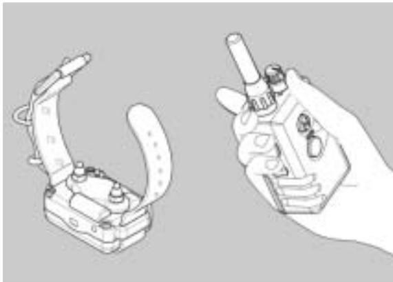
1. To activate the *dogtra* 180NCP Woodgrain Finish, place the red dot on the back of the transmitter to the red dot on the collar. Hold the two red dots together for a moment until the LED indicator light comes on. The indicator light will blink every two seconds showing the unit is charged and ready to use. (If the indicator light emits a red color, the batteries need to be charged.)
