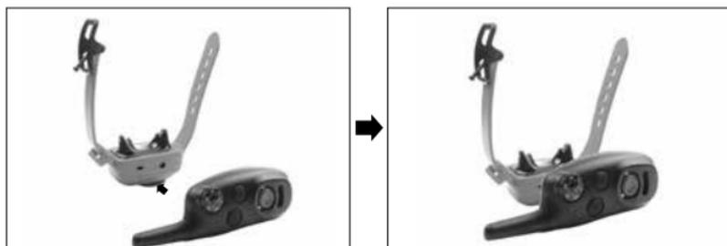
To turn the receiver on, place the red dot on the back of the handheld transmitter to the red dot on the receiver. Hold the two red dots together for a moment until the LED light on the receiver comes on.
