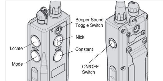
The transmitter for the ***dogtra 2500 T&B Series*** has five buttons (two on the face of the transmitter, two on the left side, and one on the right side.).
