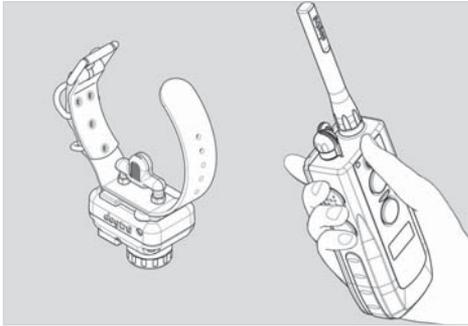
1. To activate the receiver/collar, place the red dot on the back of the transmitter to the red dot on the receiver/collar. Hold the two red dots together for a moment until the LED light on the receiver/collar comes on. The indicator light will come on for a moment then blink once every 4 seconds, showing that the collar is ready to use (If the indicator light is red, or if there is only 1 bar showing on the battery icon on the LCD transmitter screen, the unit needs to be charged.).
