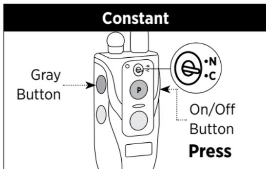
Move the toggle switch down for "C." Hold down the on/off button and the gray stimulation button.
