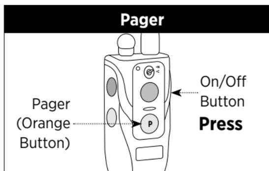
Hold down the on/off button and the orange Pager button. The toggle switch position does not matter.
