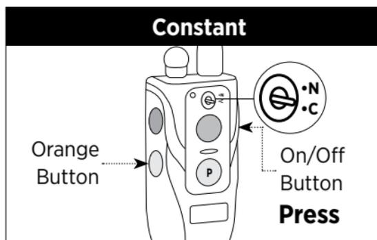
Move the toggle switch down for "C." Hold down the on/off button and the orange stimulation button.
