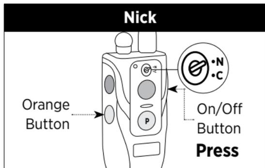
Move the toggle switch up for "N." Hold down the on/off button and the orange stimulation button.
