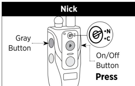
Move the toggle switch up for "N." Hold down the on/off button and the gray stimulation button.
