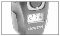
The LCD screen indicates the stimulation level on the screen ranging from (0-127). The battery life indicator shows:
