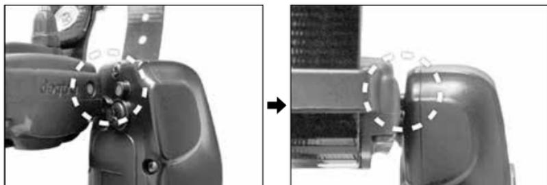
To turn on the receiver, place the red dot on the back of the transmitter to the red dot on the receiver. Hold the two red dots together for a moment until the LED light on the receiver comes on.
