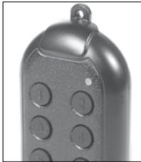
4. To make sure that the transmitter is working properly, press one of the buttons to see if the LED indicator light shows up green.
