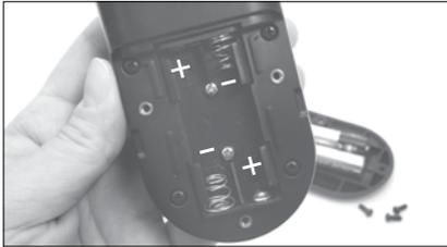
2. Replace the batteries with two AAA 1.5V alkaline batteries. Check that the batteries match the polarity indicated on the battery holder.
