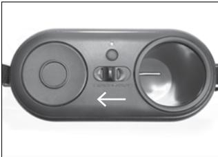
1. Put the Launcher/Dropper Mode Switch in the launch mode.
