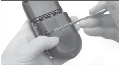
3. Place the battery cover back into place and use a screwdriver to tighten the screws back on.
