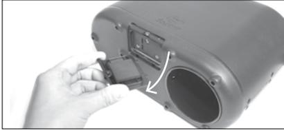
2. Carefully take out the battery holder and replace the batteries in the holder with six AA 1.5V alkaline batteries.
