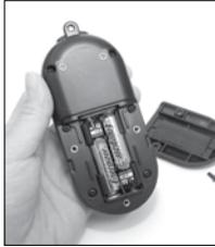
1. Using a screwdriver, remove the 3 screws on the battery cover on the back of the transmitter.
