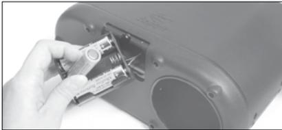
3. Before closing the battery cover, please make sure that the battery holder is properly placed into the battery compartment. Place the battery cover over the battery compartment and use a screwdriver or coin to tighten the screw back on.
