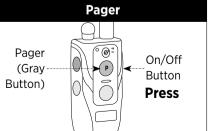
Hold down the on/off button and the gray Pager button. The toggle switch position does not matter.
