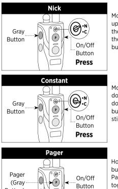
Move the togale switch up for "N." Hold down the on/off button and the gray stimulation button
