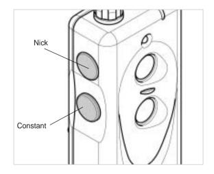
The transmitter for *dogtra* 1800NC has two buttons. The top is the Nick button and the bottom is the Constant button.
