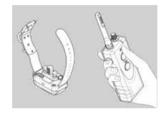
1. Turn the collar on by pressing the button on the back side of the collar receiver. The indicator light will come on for a moment then blink once every two seconds, showing that the collar is ready to use. (If the indicator light is red, the batteries need to be charged.) Place the test light on the contact points of receiver and hold it there.
