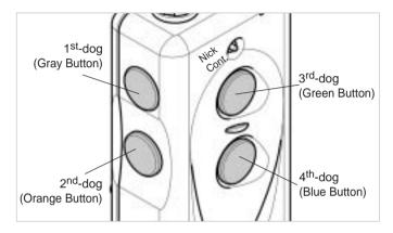
**The transmitter for the** *dogtra* **1804NC has four buttons;** The Gray (1<sup>st</sup> dog) button corresponds to the receiver with the black collar strap. The Orange (2<sup>nd</sup> dog) button corresponds to the receiver with the orange collar strap. The Green (3<sup>rd</sup> dog) button corresponds to the receiver with the green collar strap. The Blue (4<sup>th</sup> dog) button corresponds to the receiver with the blue collar strap.
