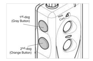
The transmitter for the *dogtrd* 1802NC has two buttons; The 1802NC has two buttons on the side of the transmitter. The gray button corresponds to the receiver with the black collar strap and the orange button corresponds to the receiver with the orange collar strap. The toggle switch at the top of the transmitter allows you to choose between Nick and Constant type of stimulation.
