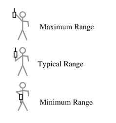
If your finger touches the antenna near the dial on the top of the transmitter, the actual range may be reduced, while you push the button on the transmitter
