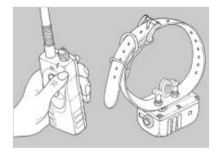
1. Turn the power switch on by pressing the button on the end of the collar receiver for one second. The indicator light will come on for a moment then blink once every two seconds, showing that the collar is ready to use. (If the red indicator light emits a double blink every two seconds, the batteries need to be charged.)
