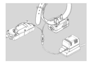
**dogtra** uses Ni-MH (Nickel-Metal-Hydride) batteries that do not set a memory and can be charged on a regular basis without harm to the battery. There is no need to completely drain the batteries between charges.
