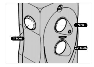
The transmitter for *dogtra* 2000 NCP has three buttons (two on the face of the transmitter and one on the side).
