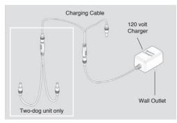
The battery charger and charging cables allow you to charge both the transmitter and receiver at the same time. The battery charger is designed for a 120-volt wall outlet (European 230-volt AC chargers and 10volt field charger for Lithium-Polymer batteries for your automobile are also available.).
