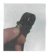
5. Lastly, thread the smaller green holder onto the stud, use the Allen wrench to tighten.
