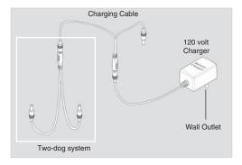
The battery charger and splitter cables allow you to charge both the transmitter and receiver/collar at the same time. The battery charger is designed for a 120volt wall outlet. (European 230-volt AC chargers and 12-volt car chargers for Ni-MH batteries are also available)
