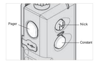
The transmitter for *dogtra* **175***NCP* has three buttons (two on the face of the transmitter and one on the side).
