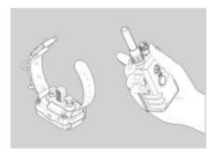
1. To activate the *dogtra* 175 NCP, place the red dot on the back of the transmitter to the red dot on the collar. Hold the two red dots together for a moment until the LED indicator light comes on. The indicator light will blink every two seconds showing the unit is charged and ready to use. (If the indicator light emits a red color, the batteries need to be charged.)
