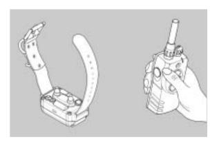
1. Turn the collar on by pressing the button on the back side of the collar receiver. The indicator light will come on for a moment then blink once every two seconds, showing that the collar is ready to use. (If the indicator light is red, the batteries need to be charged.) Place the test light on the contact points of the receiver and hold it there.
