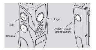
The transmitter for the **dogtrd** SUREstim HODH single dog unit has four buttons (one on the face of the transmitter, two on the left side and one on the right side).
