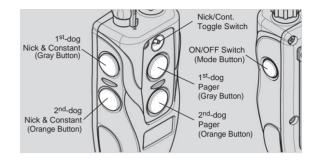
The **dogtra** SUREStim TIDEH two-dog unit has five buttons and a toggle switch on the transmitter. (Two on the face of the transmitter, two on the left side, and one on the right side.)
