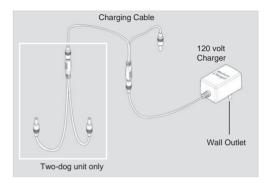
The battery charger and charging cables allow you to charge both the transmitter and receiver at the same time. The battery charger is designed for a 120-volt wall outlet. (European 230-volt AC chargers and 12-volt car chargers for Ni-MH batteries are also available)
