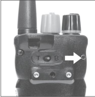
The transmitter for the T&B DUAL has seven buttons (three on the face of the transmitter, three on the left side, and one on the right). You can use the Setting Toggle Switch on the back of the transmitter to change from **T** (Training Setting) to **B** (Beeper Setting).
