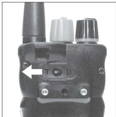
You can use the Setting Toggle Switch on the back of the transmitter to change from **B** (Beeper Setting) to **T** (Training Setting). The Training Setting offers Nick/Constant, HPP Vibration, and Locate functions.
