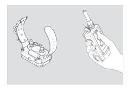
1. To activate your *dogtrd* 280NCP Platinum Series place the red dot on the back of the transmitter to the red dot on the receiver/collar. Hold the two red dots together for a moment until the green colored LED indicator light comes on. The indicator light will blink every 2 seconds showing the unit is charged and ready to use (If the indicator light emits a red color, the batteries need to be charged.).
