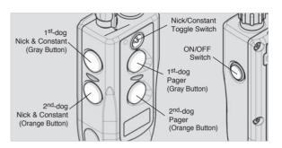
The **dogtrd** 282NCP Platinum two-dog unit has five buttons and a toggle switch on the transmitter. Two on the face of the transmitter, two on the left side, and one on the right side.
