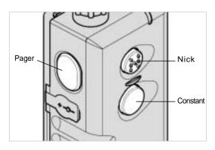
The transmitter for *dogtra* 180NCP Woodgrain Finish has three buttons (two on the face of the transmitter and one on the side).
