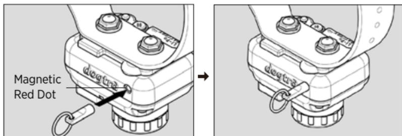
To turn on the STB BEEPER COLLAR or STB HAWK COLLAR, place the activation magnet on the magnetic red dot on the system. Hold them together for a moment until the LED light comes on. The system will play a melody and then beep twice when it is turned on.
