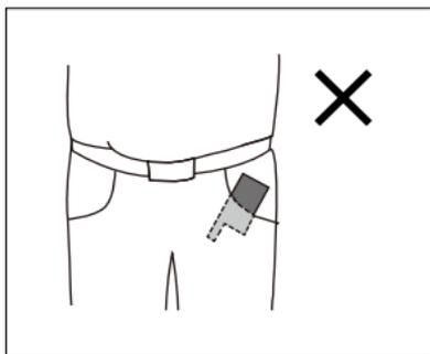
Do not place the handheld transmitter with the antenna touching your body or facing downwards.
