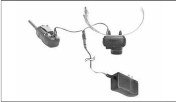
The Dogtra 2700T&B uses a lithium polymer battery. Recharge the unit if the indicator light is red or does not come on, the transmitter LCD shows only 1 bar on the indicator, or the system will not stay on when any button is pressed.
