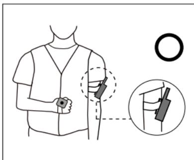
Carry the handheld transmitter with the antenna facing away from you.
