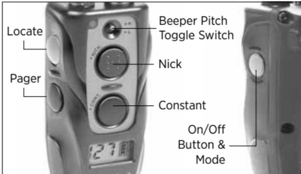
The transmitter for the 2700T&B has five buttons (two on the face of the transmitter, two on the left side, and one on the right side).
