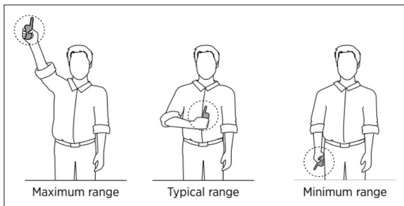
The range on the 2700T&B is reduced when the handheld transmitter's antenna is covered or in contact with your body. Refer to the following carrying methods for optimal range.
